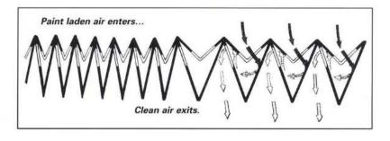
All Com-Pleat filters are designed with our unique Reverse Memory Pleats which naturally cause the filter to expand to 8 pleats per foot. This allows for maximum air flow and overspray loading capacity while eliminating the wasteful bunching seen in other accordion style filters.
